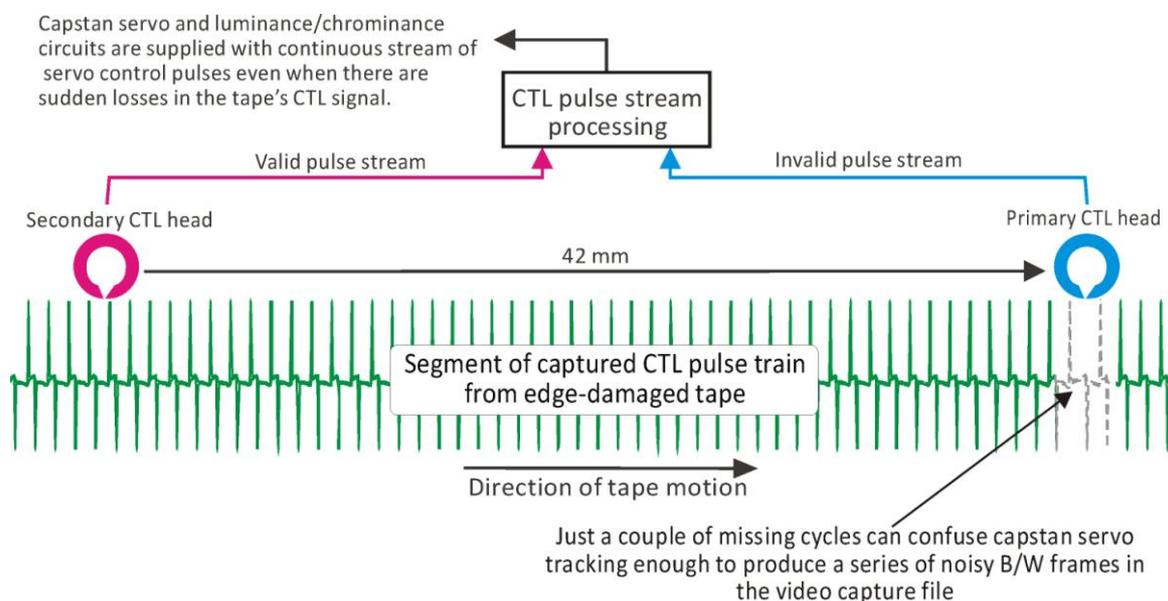
*Figure2. Principle of two-point CTL signal pick-up.*
