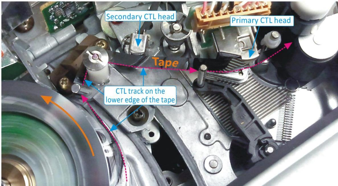
Figure 1. Secondary CTL head added to Panasonic AG-7330.
